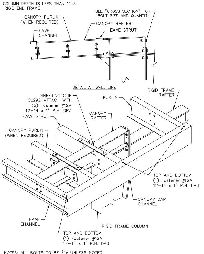
NOTES: ALL BOLTS TO BE  $\frac{1}{2}$ " $\phi$  UNLESS NOTED. FOR REQUIRED LENGTH REFER TO GRIP TABLE ON CUSTOM ERECTION DRAWINGS.
